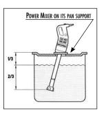
Always make sure that the bell is sufficiently immersed to avoid splashing and that the air vents of the motor unit does not come into contact with any liquid.
