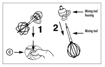
To release the mixing tool from its housing, simply press the button **C**. All that then remains to be done is to remove the housing from the motor unit.
