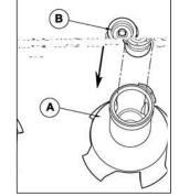
Direct the ears of cartridge **B** in order to be aligned with the groove of the bell **A**. Push the cartridge with the hand in the direction of arrow, then clip on into the bell thanks to the knife dismantling tool.
