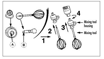
Line the flat side of the mixing tool **B** up with the flat side of the housing **A**.
